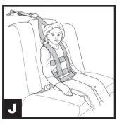
This vest requires use of a tether. The vehicle's safety belt goes through loops near the hips.
